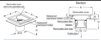
Inoxsystem® IDrain 3078 - Floor drain with standard cover and per satin finish edges - horizontal outlet - removable filter and odor trap Flow rate В D Removable Art.: Width Ø Outlet Length cover 30785010 100 80 50 12 Standard 30787510 100 75 80 25 Standard 30785015 150 80 50 12 Standard 75 30787515 150 80 25 Standard 3078AR On request 70/80 50/75 12/25 Standard Dwg. No. 3078 - Made of: Aisi 304 stainless steel, 2 mm thick - Aisi 316 on reque
