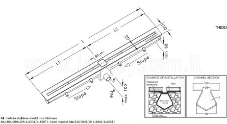
All made in stainless steel 2 mm thickness Alsi 304/304L(EN 1.4301/1.4307) - Upon request Alsi 316/316L(EN 1.4401/1.4404)
